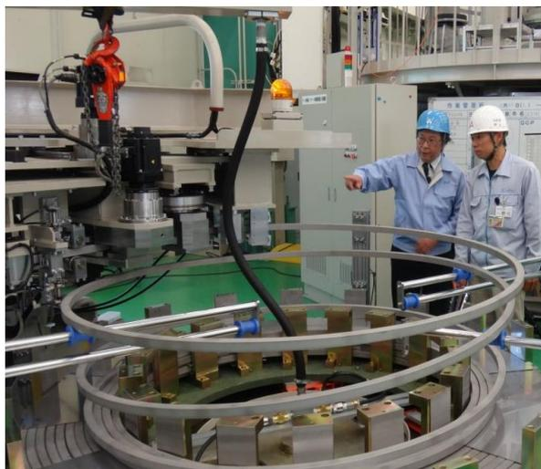
Manufacturing of CS1 module; under 2<sup>nd</sup> OP winding
