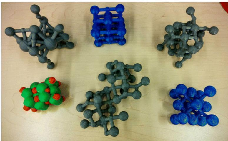
3D printed unit cells. Top image (from left to right): fluorite, tetragonal spinel, and rock salt. Bottom image (from top left clockwise): perovskite, rock salt, tetragonal spinel, fluorite, corundum, and space-filling tetragonal spinel featuring dual atom color.
