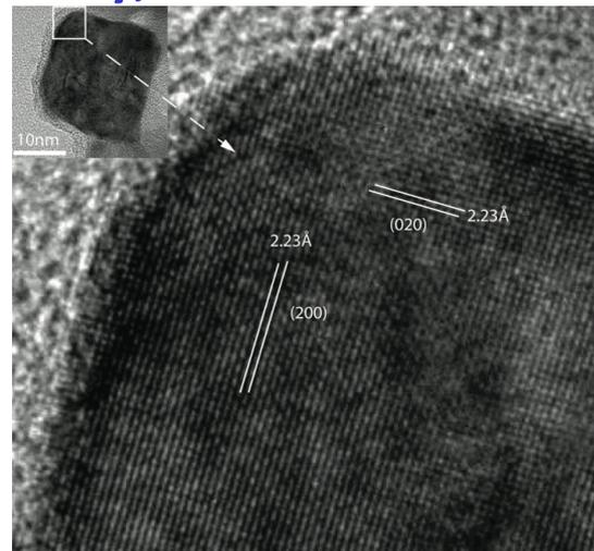
High-resolution transmission electron microscope imaging of a nano Cu(I) oxide crystal with cube shape
