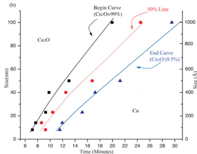
Time size reduction diagram constructed from the reduction profile
