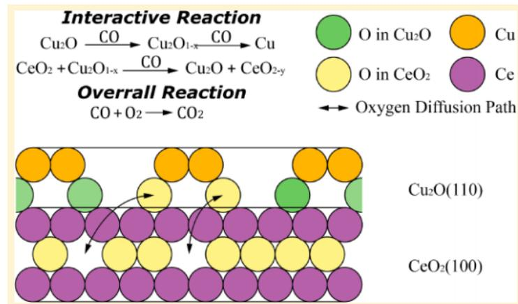
Interactive reaction takes places when  $\text{CeO}_2$  is partially reduced by lending oxygen to prevent  $\text{Cu}^+$  from reducing
