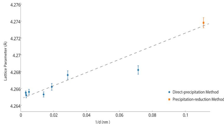
Increasing lattice parameter as Cu<sub>2</sub>O crystals size decreases.
