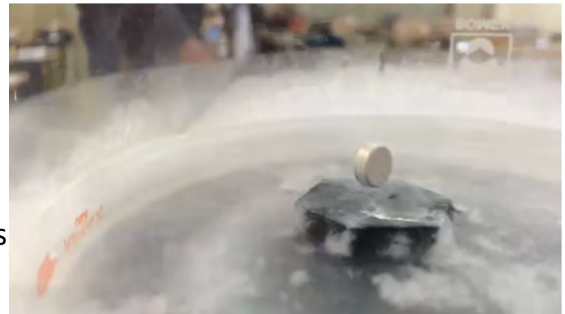
Levitation of a spinning strong magnet on top a cooled single crystal superconductor.
