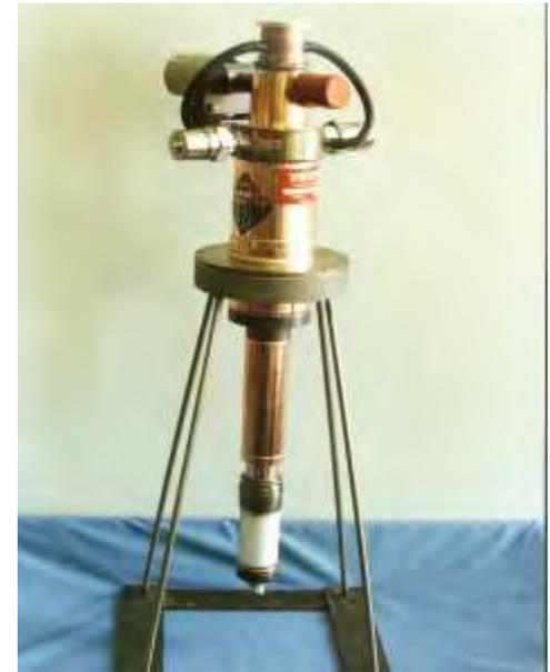
10 kW, 28 GHz gyrotron
