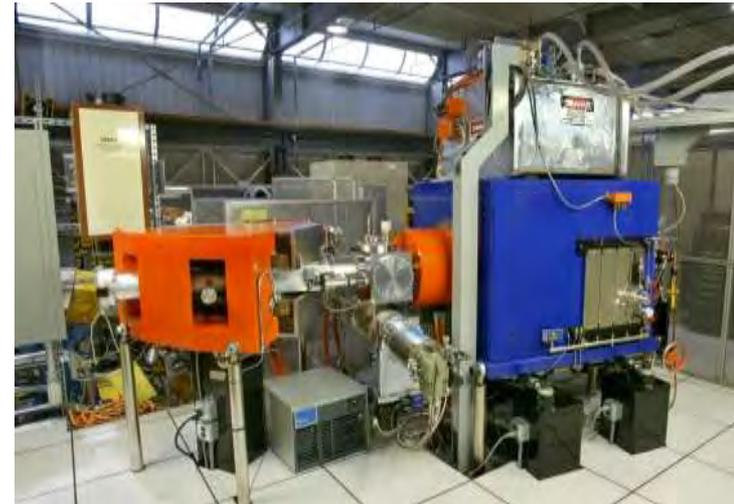
Aluminum plasma chamber for high power operation with incorporated tantalum x-ray shield
