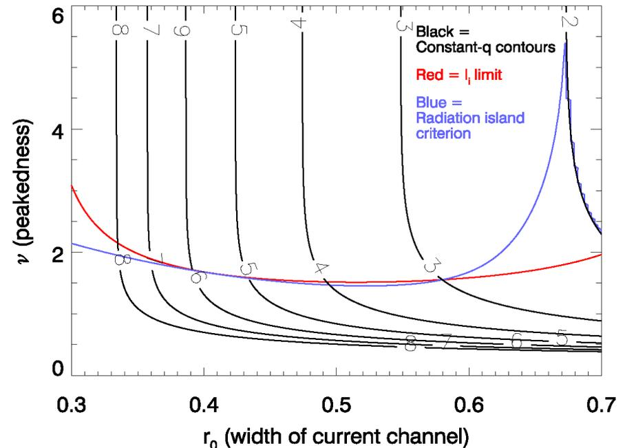
Contour plot of the total plasma current (black) as a function of the profile parameters  $\nu$  and  $r_0$ . Also shown in the plot are the contour of the current profile peaking at the density limit and the best fit contour of the radiation driven island criterion
