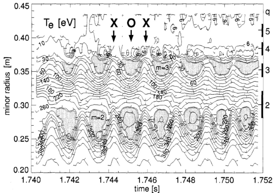
FIG. 2. Reconstruction of coupled (2,1) and (3,1) islands from  $T_e$  measurements in a time interval during current profile contraction between two minor disruptions. Islands recognized by regions of flat  $T_e$  are marked by shaded areas. While the (3,1) island grows, the (2,1) island shrinks.  $q(r)$  is derived from equilibrium reconstruction at  $t = 1.75$  s with radial uncertainties indicated.
