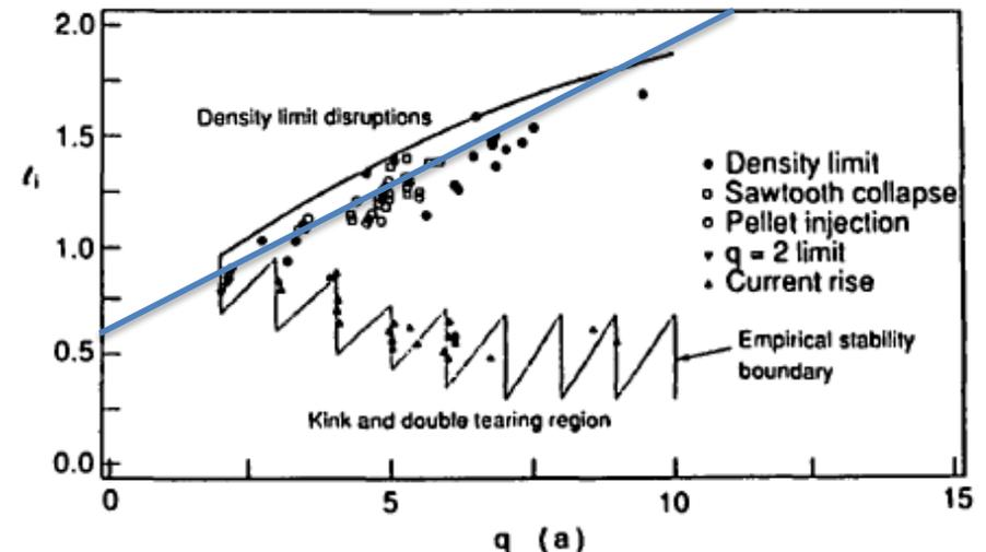
FIG. 6. Empirical stability diagram for JET, showing the  $l_i$ - $q$  plane. The lower boundary (dotted) indicates the stability boundary for rotating MHD modes during the current rise. The upper boundary (solid) indicates the region where major disruptions occur. The symbols indicate the onset of quasi-stationary modes in various situations.
