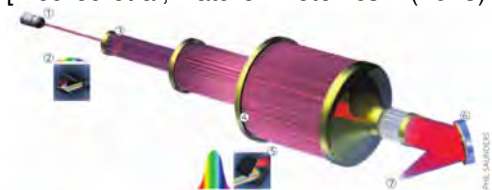
Figure 1 | Principle of a coherent amplifier network. An initial pulse from a seed laser (1) is stretched (2), and split into many fibre channels (3). Each channel is amplified in several stages, with the final stages producing pulses of \sim 1 \text{ mJ} at a high repetition rate (4). All the channels are combined coherently, compressed (5) and focused (6) to produce a pulse with an energy of >10 \text{ J} at a repetition rate of \sim 10 \text{ kHz} (7).
