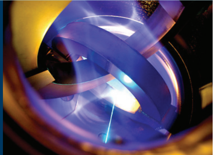
A glowing nitrogen plasma in the CNT experiment, visualizing CNT's magnetic topology. Prof. Thomas Pedersen's graphic of the Columbia Non-neutral Torus was featured in the 2006 American Physical Society (APS) Calendar.
