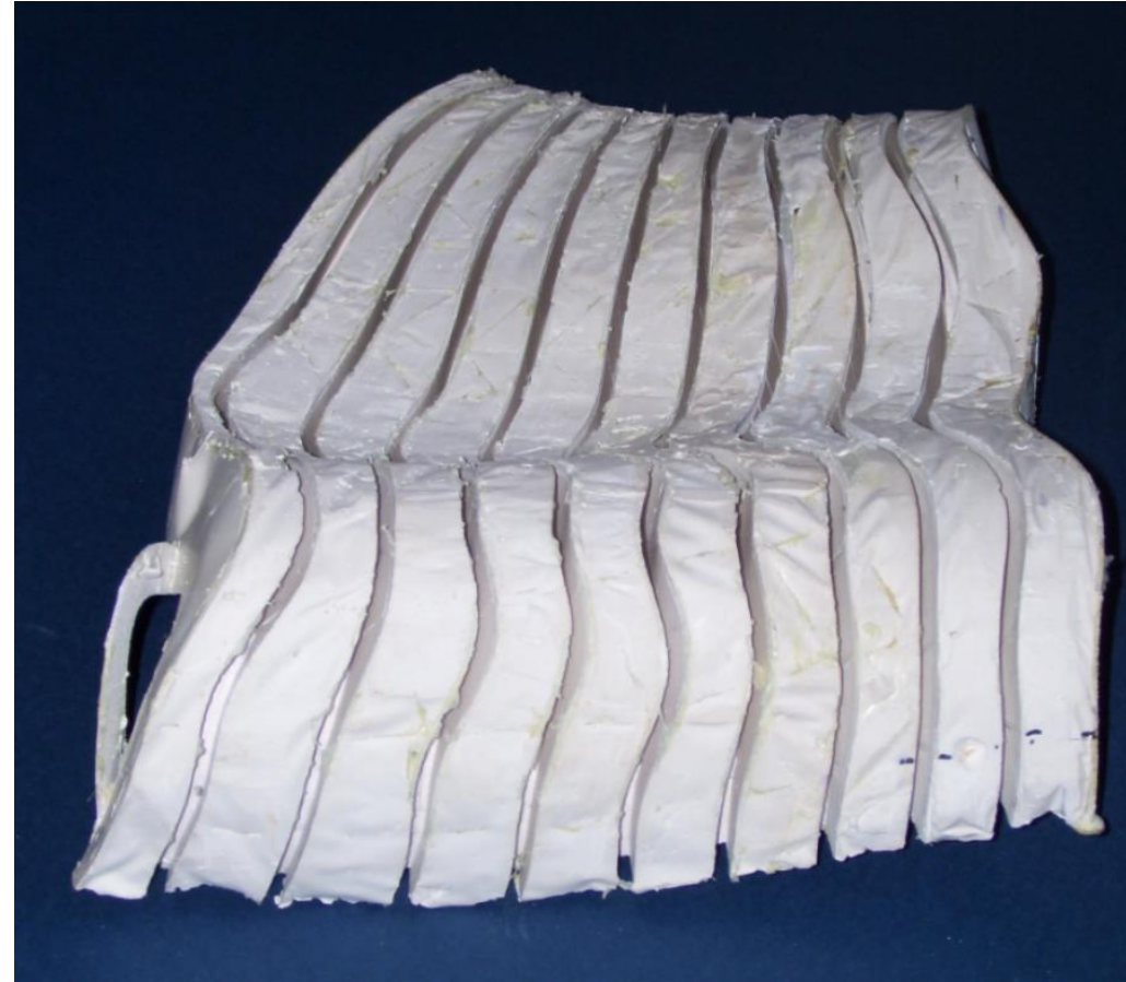
One half-sector after hard plaster moulding
