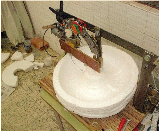
Creating the porexpan mould
