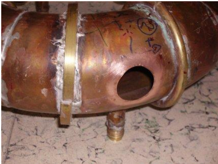
Reinforcements and opening for port
