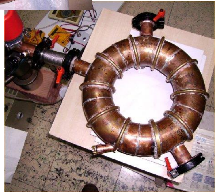
Finished vacuum vessel. 3 large ports and one small
