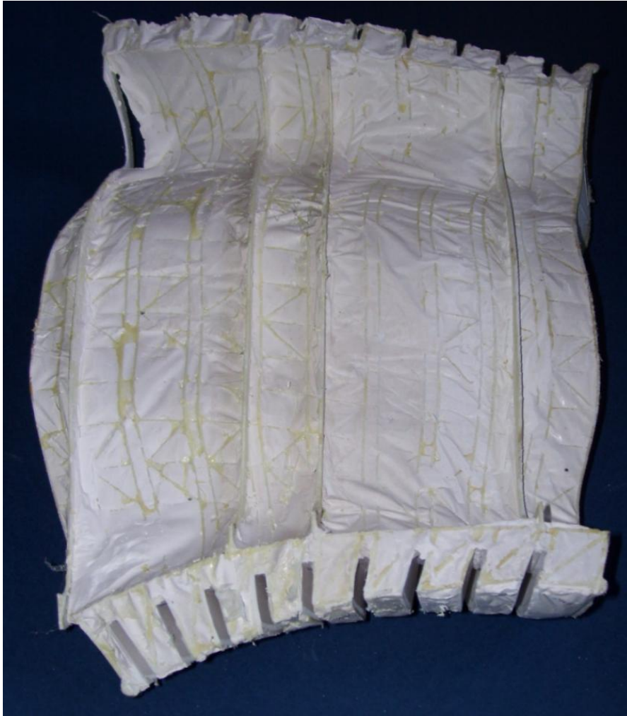
One half-sector after hard plaster moulding
